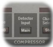
Det Input (Detector input): Main (channel 1+2), SC (channel 3+4/side-chain)
