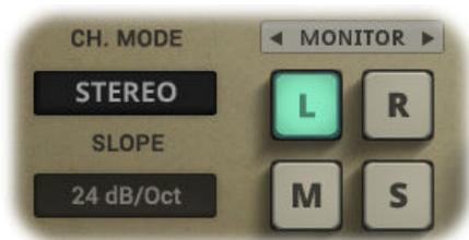
Channel mode will apply the filter only to the selected channel: Stereo, Left, Right, Mid/Sum or Side/Diff signal.
