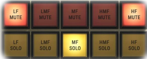
10 buttons to solo or mute the 5 frequency bands. Solo buttons override mute buttons. Click with shift left mouse button or right mouse button on any button deactivates all other buttons. This helps to quickly click through individual bands.
