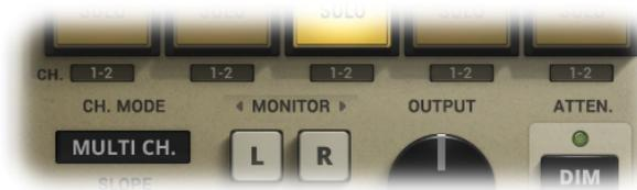
If “Ch. Mode” is set to **multi channel**, ISOL8 copies the split band to one out of five channel pairs.
