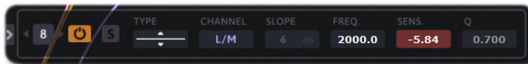
Pre-filter control the signal fed into the dynamic equalizer. You can take parts of the spectrum out (not processed by the dynamic equalizers) or boost (more processed by the dynamic equalizers).
