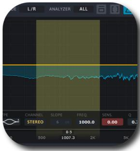
The narrow-band sweeping mode is enabled by left mouse click + ctrl key in the free area of the spectrum view. The frequency is changed by moving the mouse left/right, the Q of the filter is changed by moving the mouse up/down.
