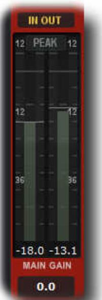
A small LED On top lids up if level goes over 0.0 dBFS. Numbers below the meters display the maximum values. Reset by mouse click.
