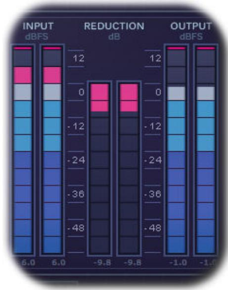
Meters for input signal (L/R Input), output signal (L/R Output) and gain reduction (L/R GR). In ISP mode True-Peak values (dBTP) are displayed otherwise peak values (dBFS).
